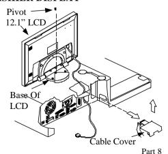
platform of the main unit till it clicks. Screw the pivot back to secure the base of the cashier display on the display platform of the main unit as in drawing below. Remove the cable cover on the display platform (same way as the instructions for CRT model) and connect the VGA connector of the 12.1" TFT LCD through the cable cover opening into the rear room. Reserve some sag in the cable so that the LCD cashier display will be allowed to turn and reinstall the cable cover.
